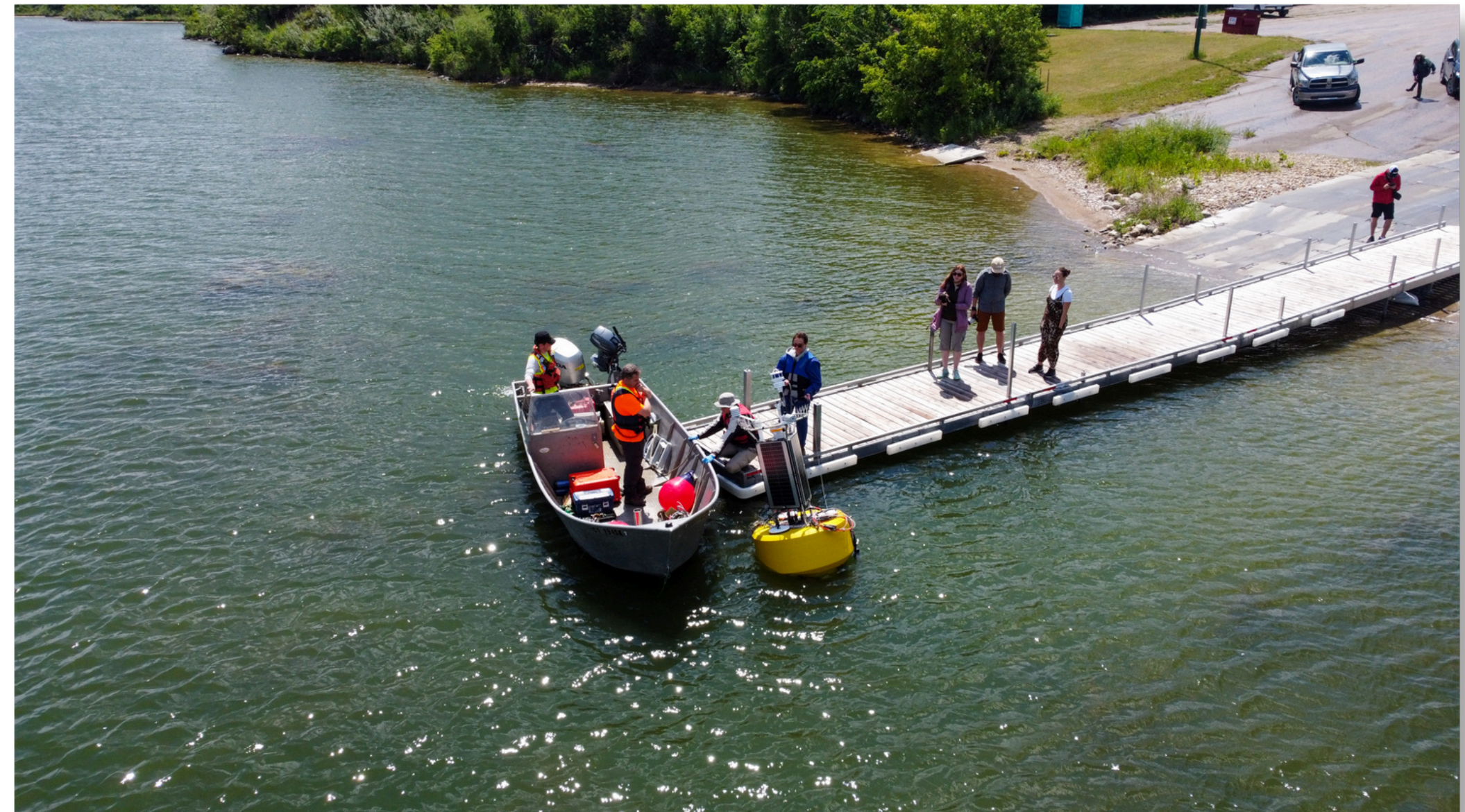
Researchers launch a real-time buoy that monitors Buffalo Pound Lake's water quality (Photo: Mark Ferguson, University of Saskatchewan)
