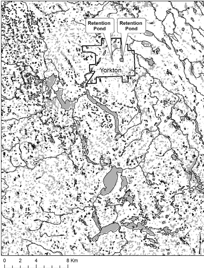
Figure 19.2 Yorkton Creek region. Gray shaded areas indicate accumulated runoff from the runoff simulation model (WDPM) output based on 110 mm of water added to the SRTM 30 m DEM. Black outlines are the surface hydrography blue lines and water bodies from the National Hydrography Network.
