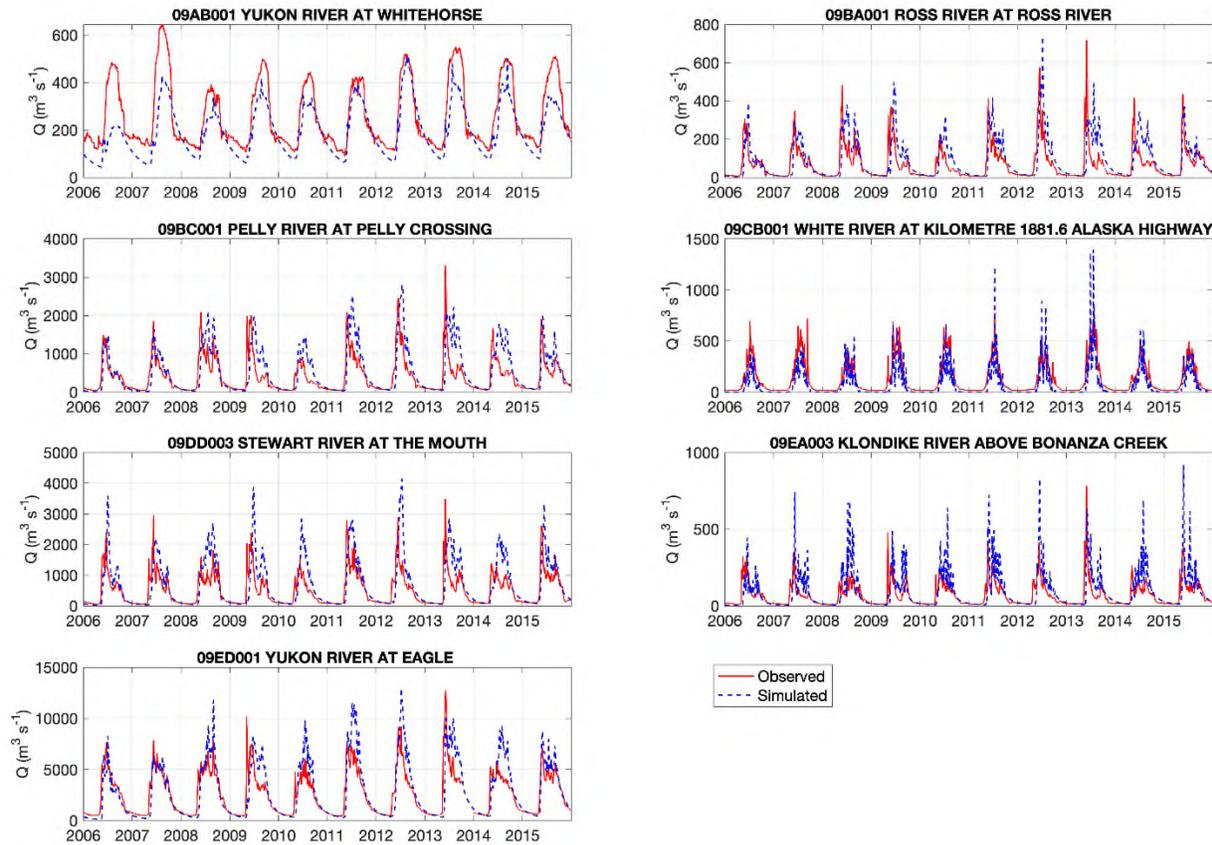
Figure 4: Comparison of RDRS-MESH vector-based model simulations against the observations from the discharge gauges of interest (Figure 1)
