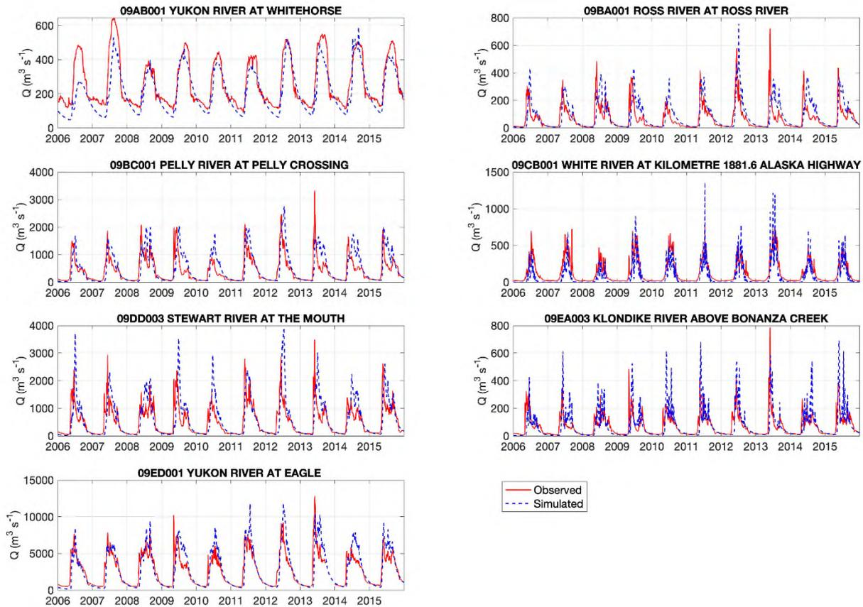
Figure 3: Comparison of GC-MESH vector-based model simulations against the observations from the discharge gauges of interest (Figure 1)
