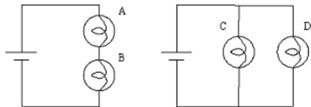
In the two circuits shown above, the batteries are identical and maintain constant voltage. The light bulbs A, B, C and D, are identical and have resistance  $R$ . Assume that the bulbs are brighter when there is more current flowing through them. Which of the following relationships correctly describe the brightness of the bulbs?
