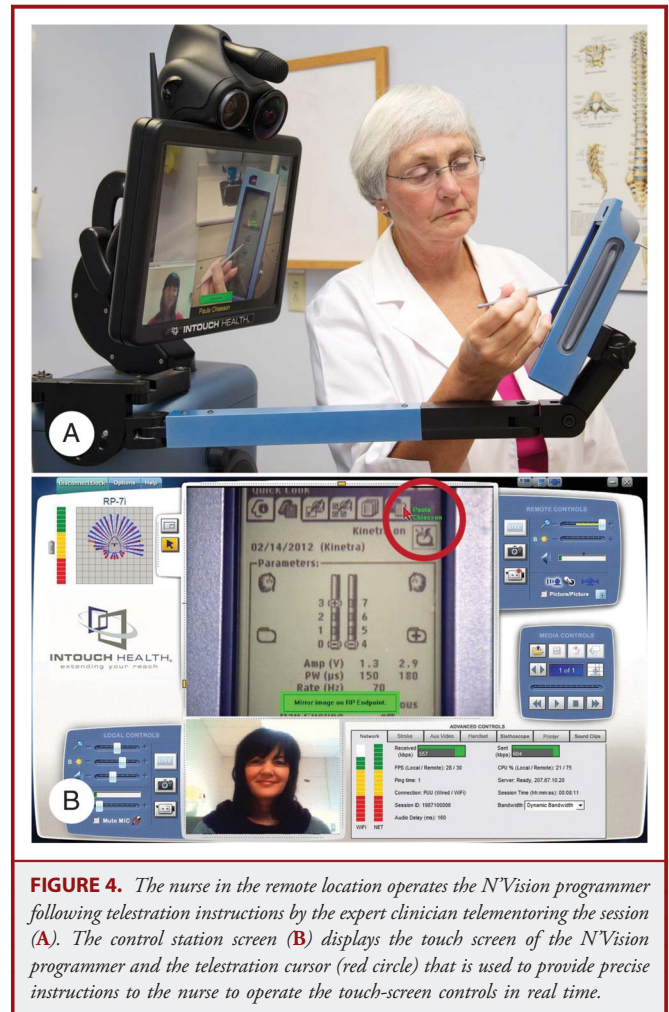
FIGURE 3. A nurse without previous experience in programming is tele-mentored, in real time, to operate the N'Vision programmer by the expert clinician (A). The control station screen gives the expert programmer full view of the patient, nurse, and the N'Vision touch-screen (B). The box on the control screen displaying the image of the expert programmer is also displayed on the head screen of the RP-7 robot.
