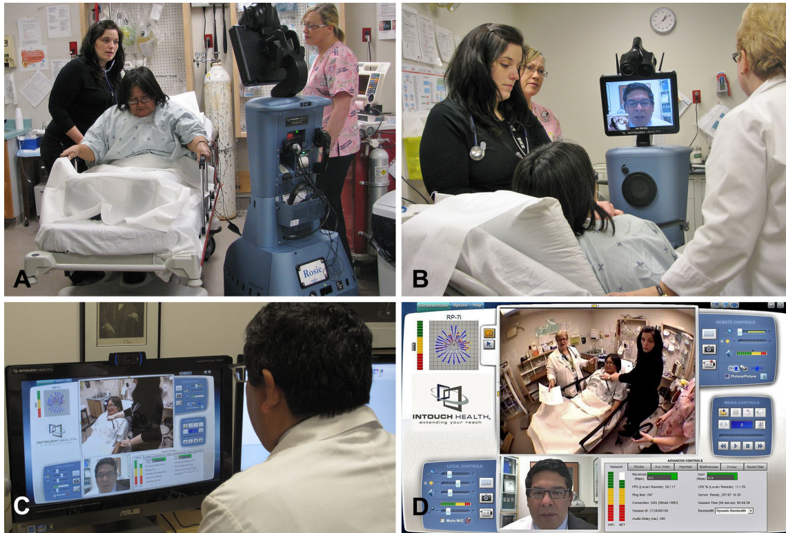
Fig. 2. Photographs of the RP-7 remote presence robot, nicknamed “Rosie” (A) at a patient’s bedside assessment; (B) the remote physician interacting with the patient and the clinical team in Nain; (C) control station used by the remote physician conducting the clinical assessment in the Nain clinic and (D) snapshot of the control screen for the RP-7 remote presence robot.
