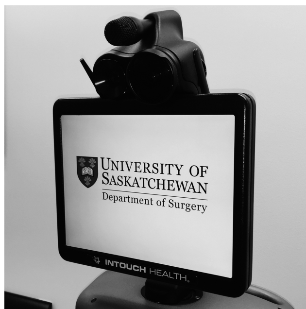
Figure 3 Close-up view of the remote presence robot's screen, two cameras and microphone (top).
