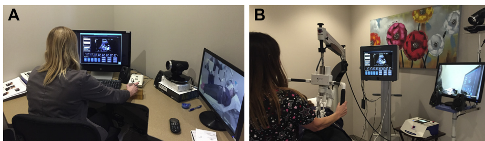
Fig. 1. (A) Sonographer site. The sonographer manipulates a mock ultrasound probe; all movements of the mock probe, including rotating, rocking, and tilting, are replicated by the scanning ultrasound probe at the patient site via a 3-degrees-of-freedom robotic arm. The sonographer can view the ultrasound machine interface, which is transmitted from the patient site and can remotely control all ultrasound machine settings. A videoconferencing system allows the sonographer to communicate with the patient and patient-site assistant. (B) Patient site. The patient-site assistant holds the frame for the 3-degrees-of-freedom robotic arm to which an ultrasound probe is attached. The patient-site assistant ensures sufficient contact between the ultrasound probe and the patient's abdomen and controls translation of the ultrasound probe based on instructions from the sonographer.
