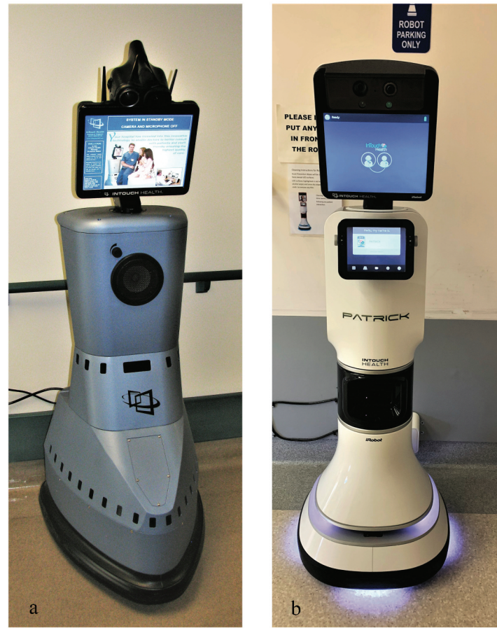
Figure 2. Remote presence technology (RPT). A) RP-7 robot; B) RP-VITA robot.
