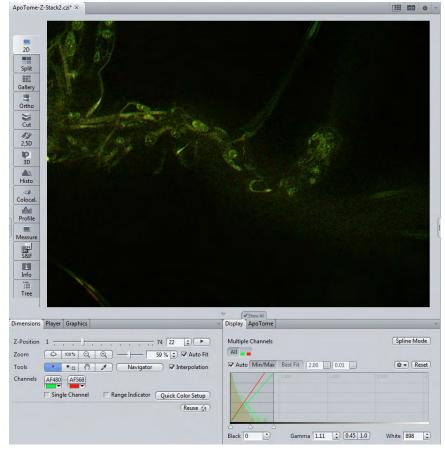
**3** Examine the result by navigating through the Z-stack using the **Z-Position** slider on the **Dimensions** tab.
