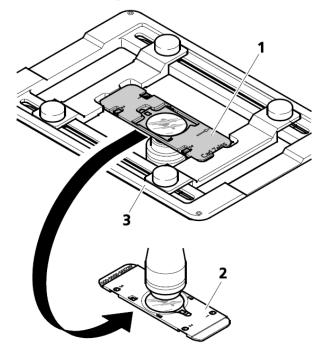
Illustration 36: Inserting a sample holder
