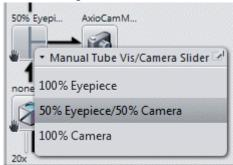
With **ZEN lite** you always control microscopes manually. After a change in the light path you therefore will immediately be asked to perform this change also on the microscope.
