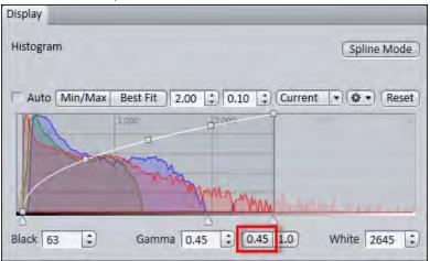
**3** Move the controls under the display curve left and right in order to directly adjust the values for **Brightness** (White), Gamma, and Contrast (Black) in the live image.
