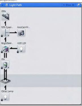
**Procedure 1** In the **Lightpath** tool set the components that you want to use for the acquisition.
