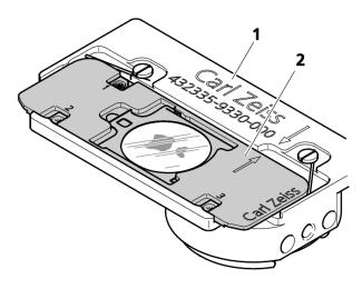
Illustration 40: Sample holder mounted in SEM adapter
