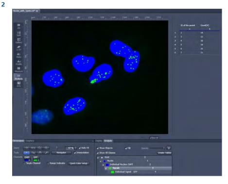
Only the number of signals of measured nuclei is displayed. Nuclei touching the frame are not taken into account.
