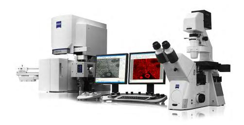
Illustration 24: SEM / LM system for correlative microscopy
