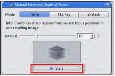
The **Central Screen Area** will be split into two parts. Right you will always see the current live image, left you will see after each new acquisition the actual calculated extended focus image.
