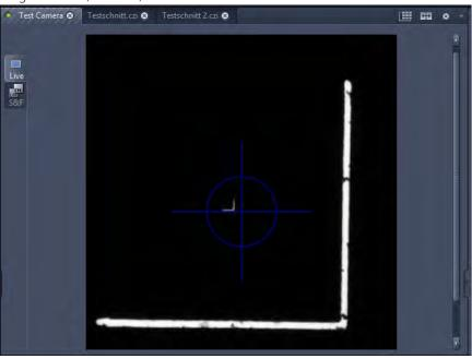
locate the marker positions we recommend to use a dry objective with low magnification (5x - 20x).
