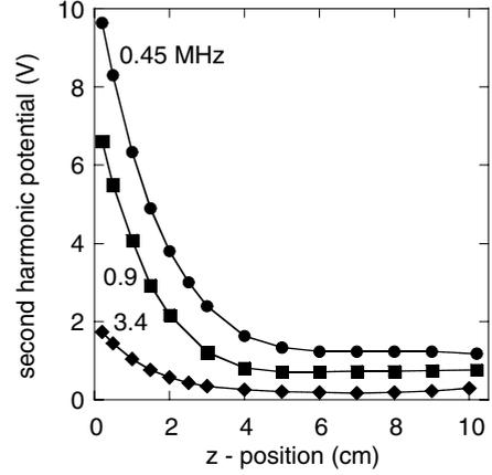
**Figure 4.** Axial distribution of the SHP for different driving frequencies.  $P = 200$  W and  $p = 1$  mTorr.
