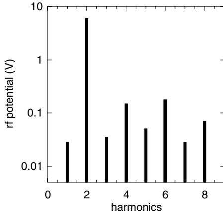
**Figure 1.** Plasma potential spectra measured in the skin layer.  $P = 200$  W,  $p = 1$  mTorr,  $f = 0.45$  MHz,  $z = 1$  cm and  $r = 4$  cm.
