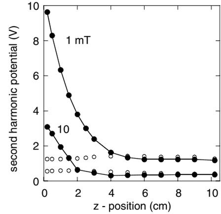
**Figure 2.** Axial distribution of the second harmonic potential for  $f = 0.45$  MHz and  $P = 200$  W. The full circles correspond to  $r = 4$  cm and the open circles correspond to  $r = 0$ .
