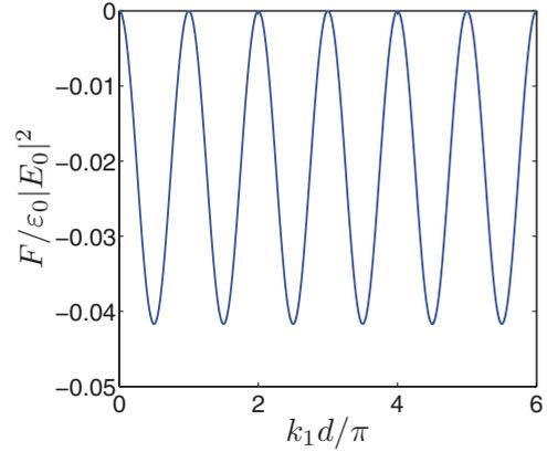
FIG. 3. (Color online) The total force on the coating film as calculated from Eq. (62);  $\varepsilon_1 = 1.5$  and  $\varepsilon_2 = 2.25$ .
